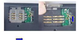
3 Put the SIM card into the holder, and turn the foil right and fasten it in place.
