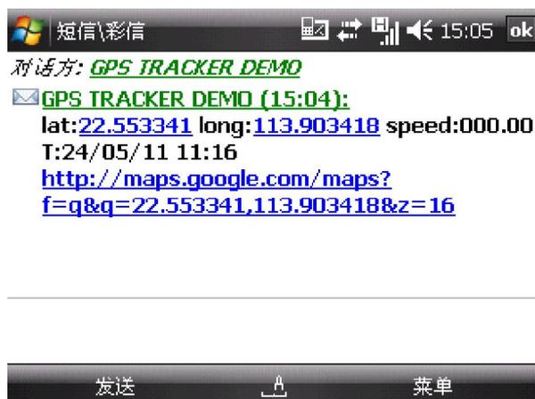
\*Tracking location, the SMS information about the lat./long. Received is the place received the GPS signal when the GPS signal is weak. Please check the time received the SMS if there are some errors of the location.
